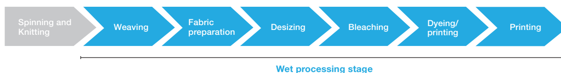
Figure 4: Flow diagram of fibre processing stage in WDF factories
